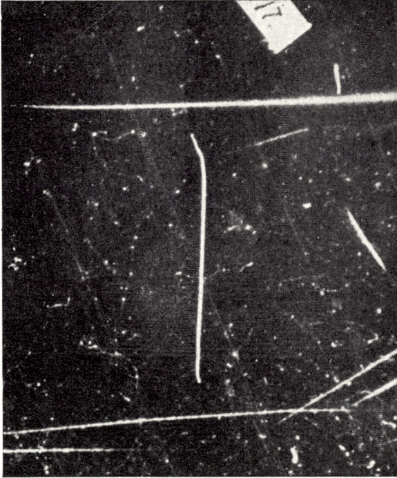
Fig. 5. Track of the long range group. Shows the characteristic bending in both ends.
