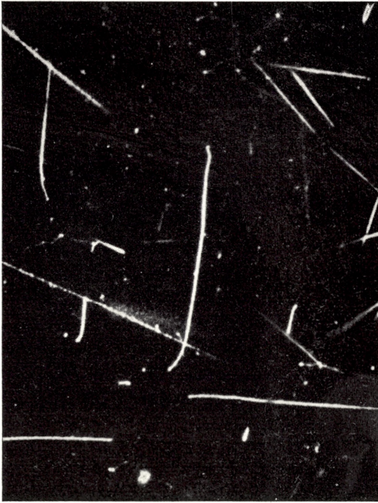
Fig. 3. Track of boron disintegration. The type of track is established by means of the characteristic feature, i. e., the fortuitous bending of both ends of the track demonstrates that the velocity is small in both ends. The track is thus produced by two ionizing particles originating somewhere in the track and moving in opposite directions.
